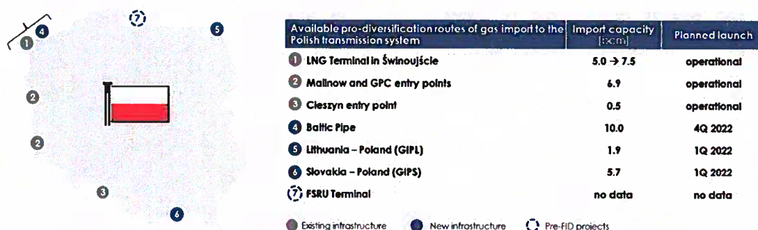
Figure 2: Existing and planned TPA entry points to the Polish transmission system.
